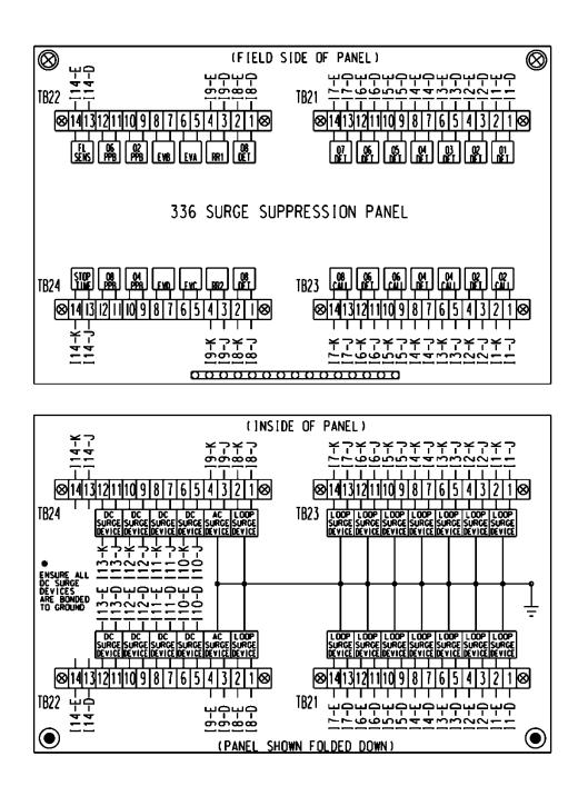
For base mounted cabinets, mount surge protection panels on the left side of the cabinet as viewed from the rear. Attach each panel to the cabinet rack assembly using bolts and make it easily removable. Mount the surge protection devices in vertical rows on each panel and connect the devices to one side of 12 position, double row terminal blocks with #8 screws. For each surge
